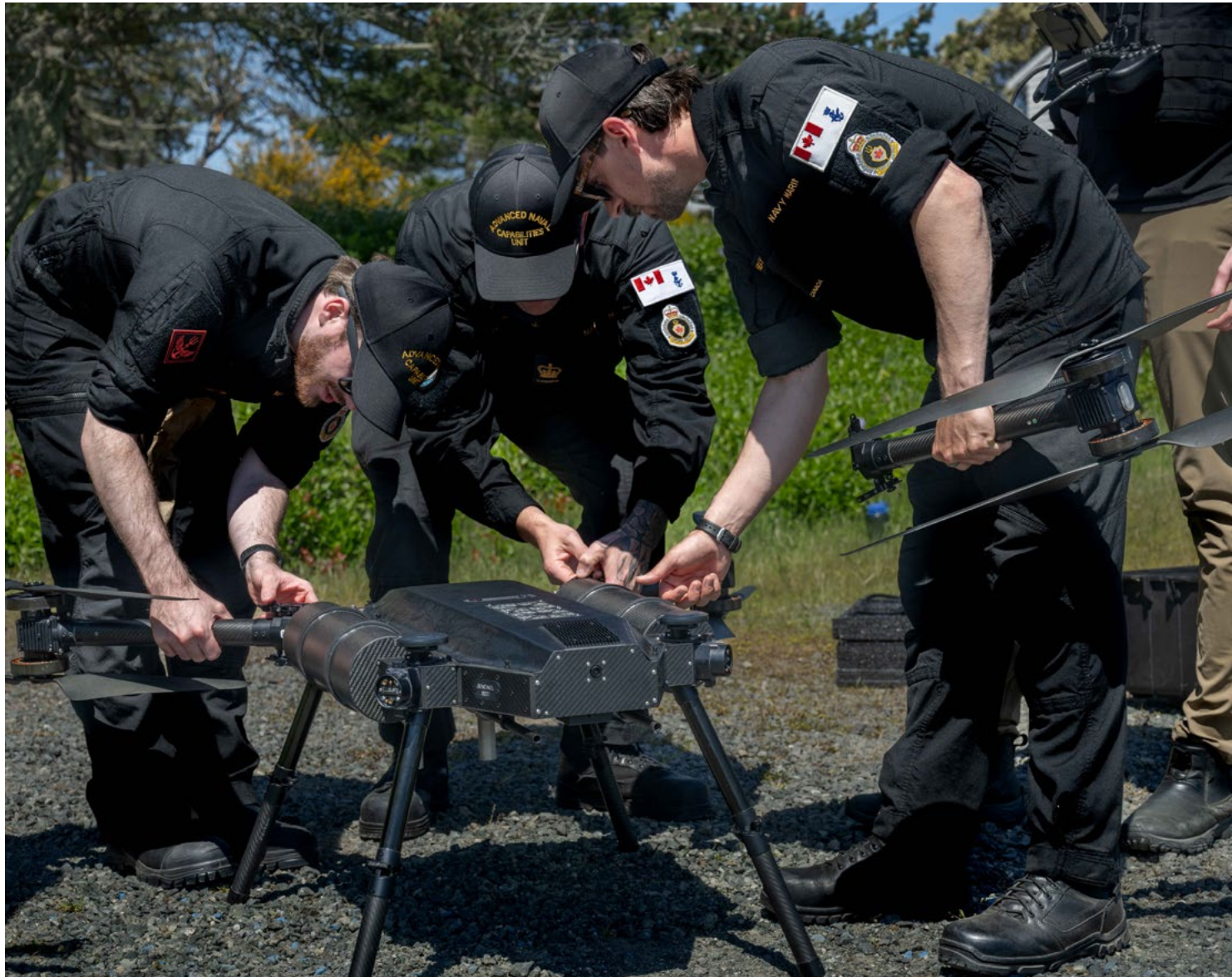
Members of the Advanced Naval Capabilities (ANC) Unit assembling a modular uncrewed aerial system.
