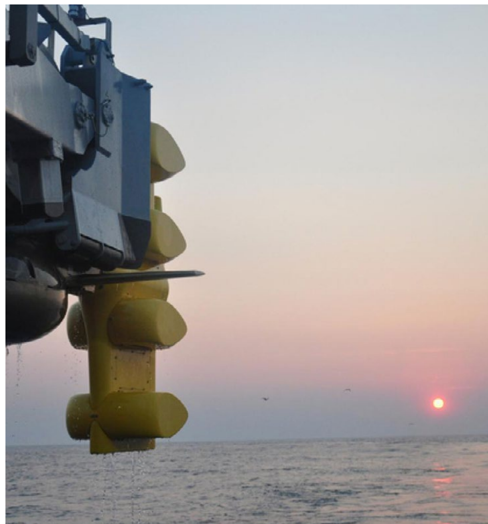
The S2087 low frequency towed array sonar.
