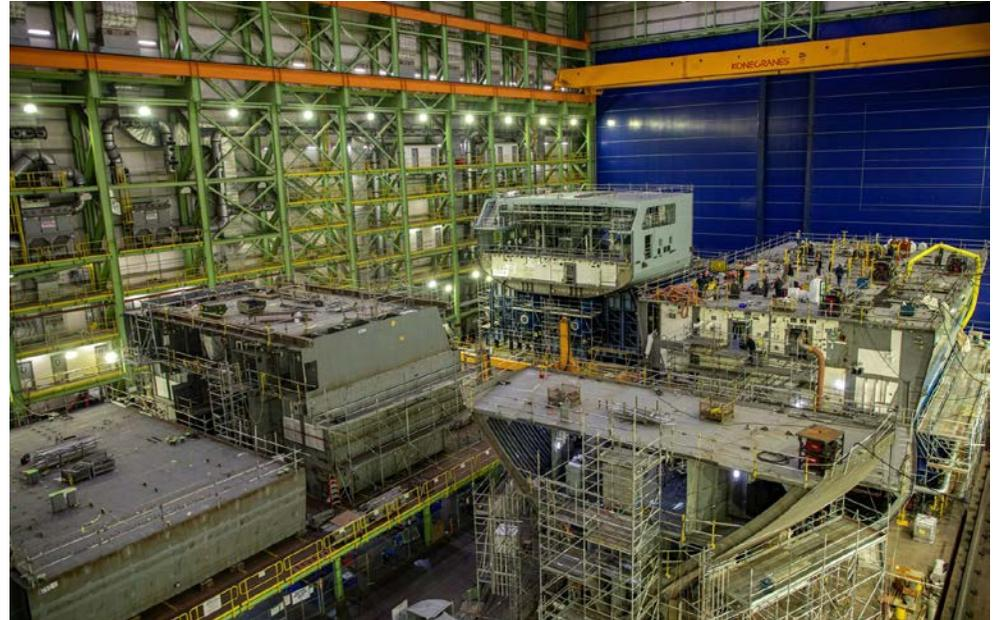
Irving shipbuilding recently shared an update on the construction of the future HMCS Frédéric Rolette from the Module Hall of the company's Halifax Shipyard. The ship's three mega blocks are currently taking shape, and will likely be moved outside to the land level this coming summer. The future HMCS Frédéric Rolette will be the fifth Arctic and Offshore Patrol Ship to be delivered to the Royal Canadian Navy.
