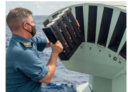
*The surface off-board passive decoy is just one component of the Halifax-class Anti-Ship Missile Defence suite.*
