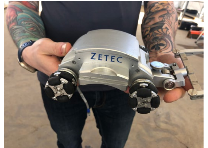
Eddyfi Technologies’ lightweight scanner can inspect hard-to-reach areas for corrosion.
