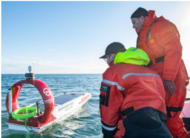
Researchers prepare to install a hydrophone on the Data Xplorer.
