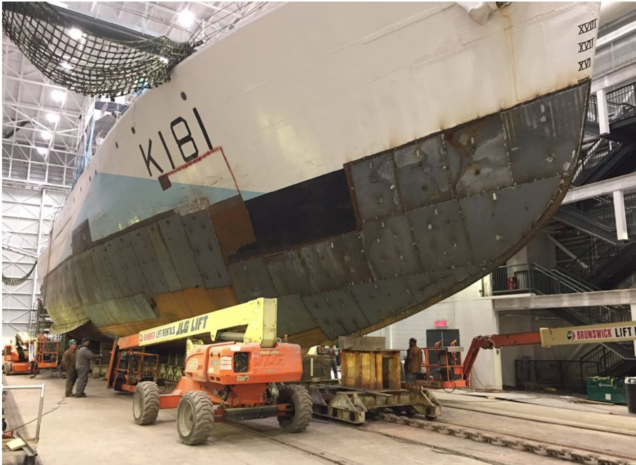
HMCS Sackville has been away from its winter berth in recent months as crews add extra plating to the underwater portion of the ship's hull, ensuring watertight integrity until permanent repairs can be made.
