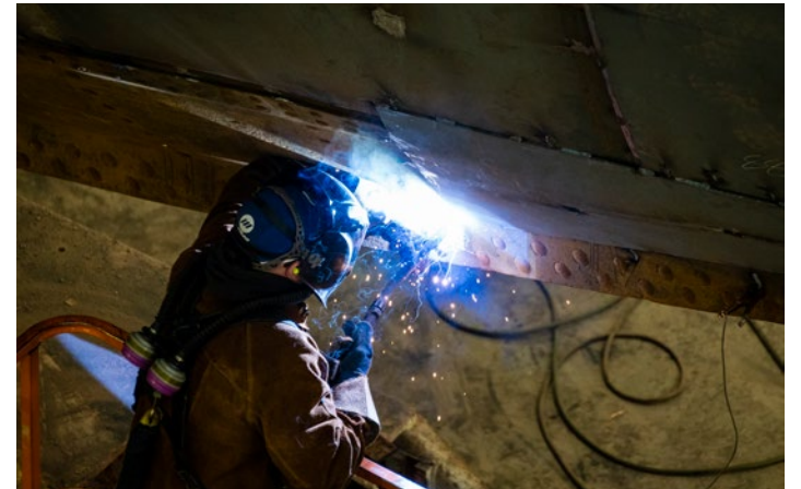
New plates are welded onto the underside of the ship inside the submarine shed at FMF Cape Scott.
