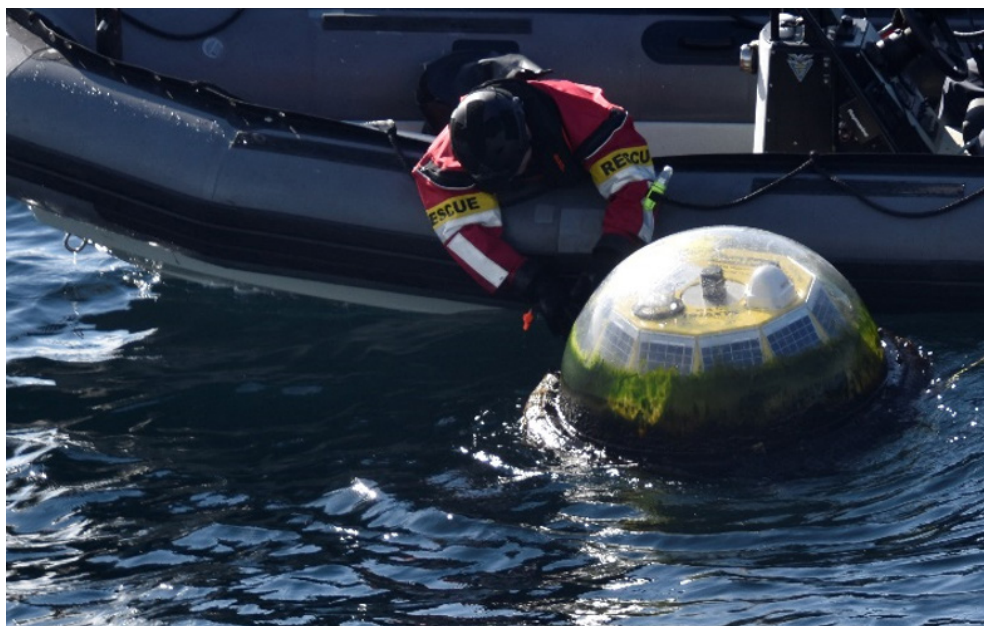
The RHIB team attached a bridle to the buoy in order to hook it to a crane and safely lift it on board.
