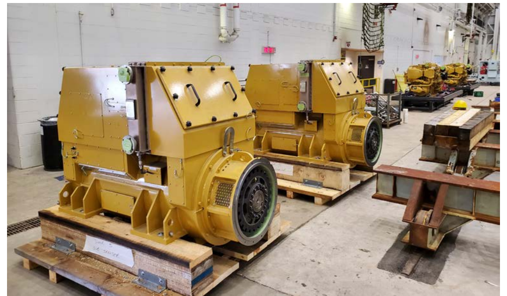
Two generators sitting on cradles in the foreground built by the Shipwright Shop, with CAT engines still in shipping bases in the background.
