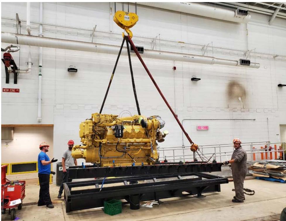
Riggers removing the engine, with steel bed attached from the shipping base.
