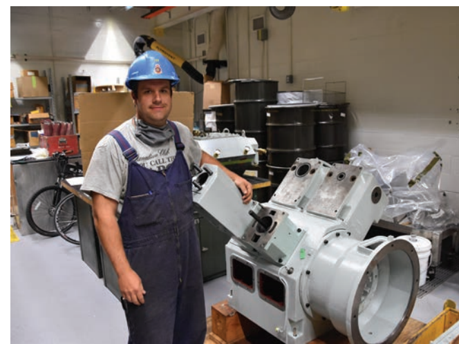
Bobby Sluggett, a Mechanical Fitter at Fleet Maintenance Facility Cape Breton, poses next to a refitted High Pressure Compressor that is ready to be put back onboard HMCS Winnipeg .
