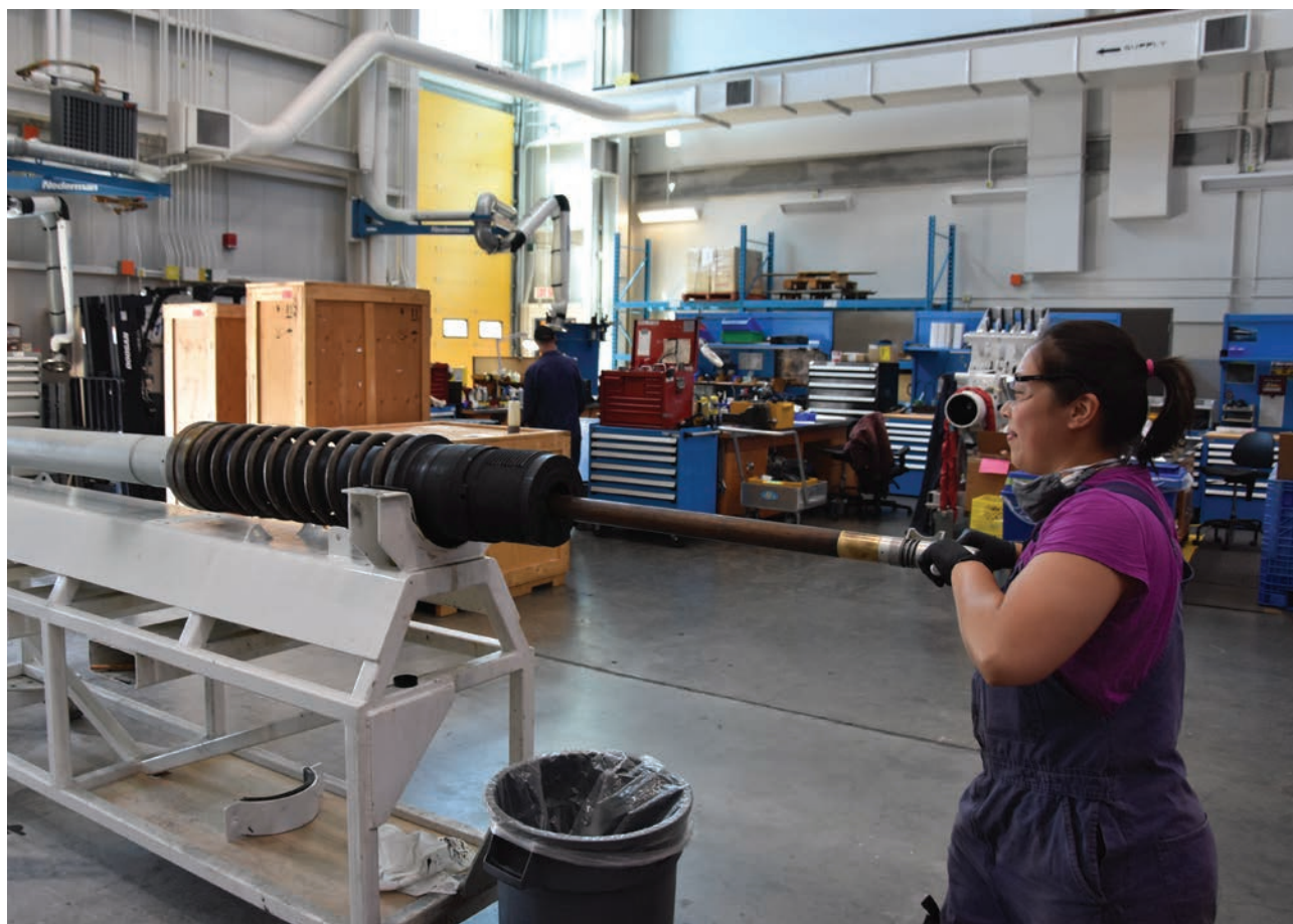
Antoniette Yap, a Millwright Apprentice at Fleet Maintenance Facility Cape Breton, cleans the 57mm barrel of HMCS Winnipeg's main gun in preparation for an inspection of Naval Ordnance.
