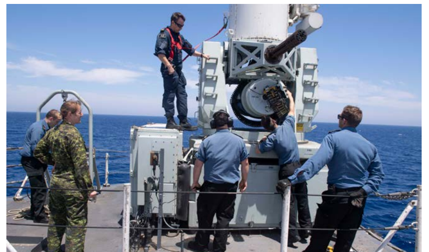
Maj Carra Greenhorn (second from left), a social worker deployed onboard HMCS Fredericton, accompanies a group of Combat Systems Engineers while they conduct post fire maintenance on the Close-In Weapon System during Op REASSURANCE in May 2020.
