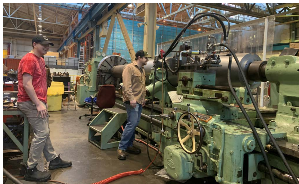
Machinists at FMF Cape Scott create a custom-made rudder shaft for HMCS Charlottetown .
