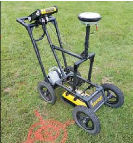
The Noggin 500 Ground Penetrating Radar, with attached GPS, is one of the tools being used to conduct a geophysical survey of the northeast corner of RA Park.
