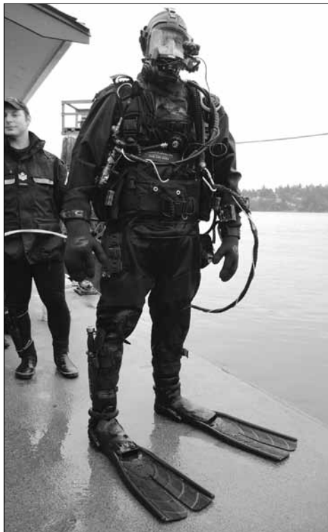
The Ultra Lightweight Surface Supply Diving System includes lightweight carbon fiber reserve and regulator tanks, a more portable surface supply system, and a much smaller umbilical cord, the long yellow hose that supplies divers with an unlimited supply of high pressure breathing gas, along with enhanced communication and sensory capability.
