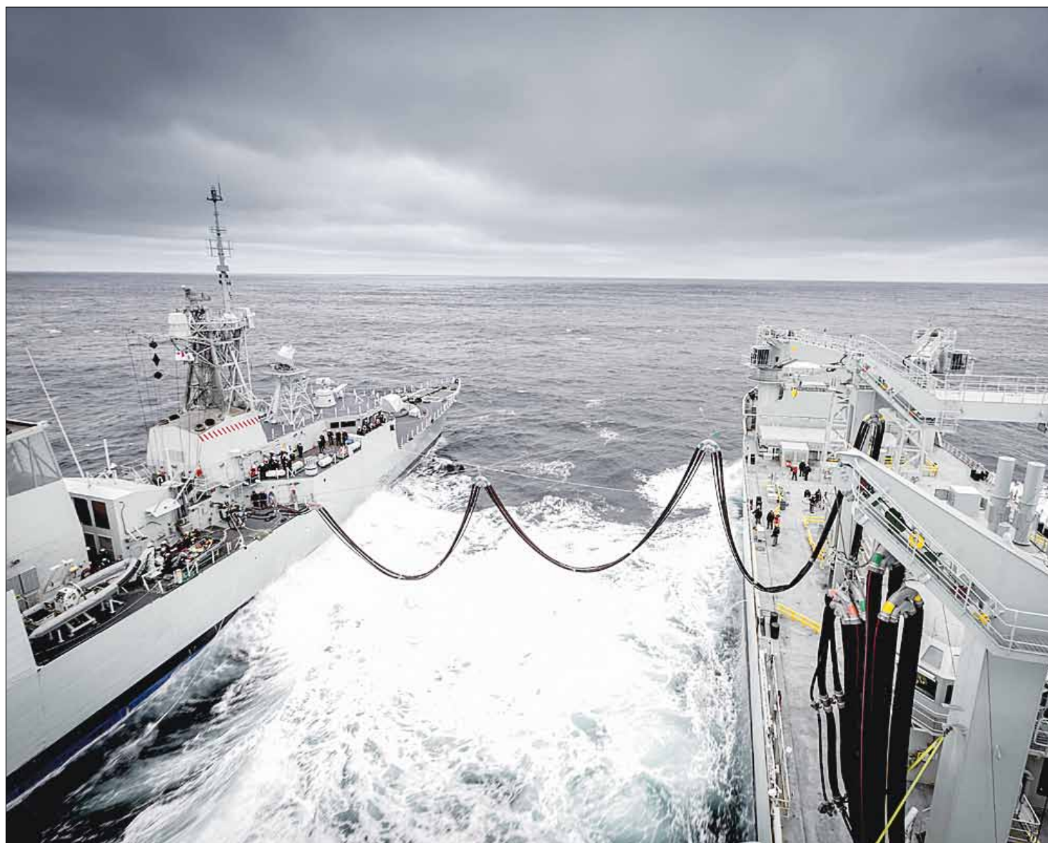
HMCS Toronto, left, and MV Asterix, connected for RAS at sea.
