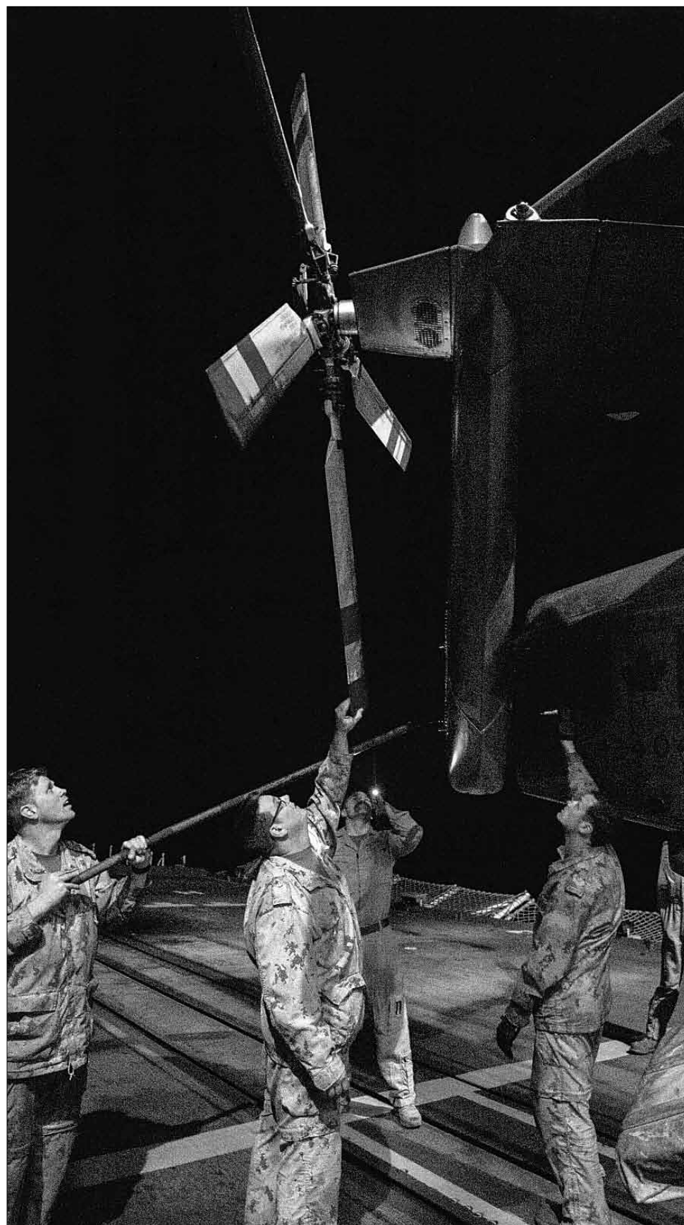
The Air Department of HMCS Charlottetown fold in the tail rotor and stow their CH-124 Sea King helicopter at the end of a flying mission during Operation REASSURANCE.
