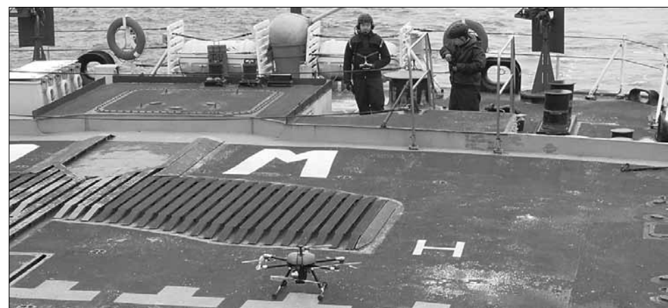
A recent scenario aboard one of the frigates featured a Sniper multi-rotor target using QTS's Universal Target Control System, which allows the operation of multiple unmanned systems from a single command centre.
